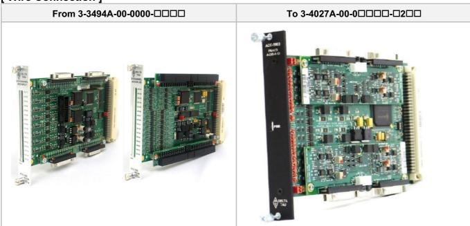
Only D-Sub option is available for ACC59E3, Terminal Block option not available for ACC-59E3
