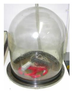
After 30 minutes stabilising at altitude the mated connectors were subjected to a voltage of 1000V AC for size 22 contacts, applied between each contact to all others. This voltage was applied at a rate not exceeding 500V per second and maintained for 60 seconds.
