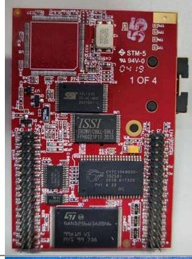
Backside of original, red PCB, showing unused component footprint in upper-left.
