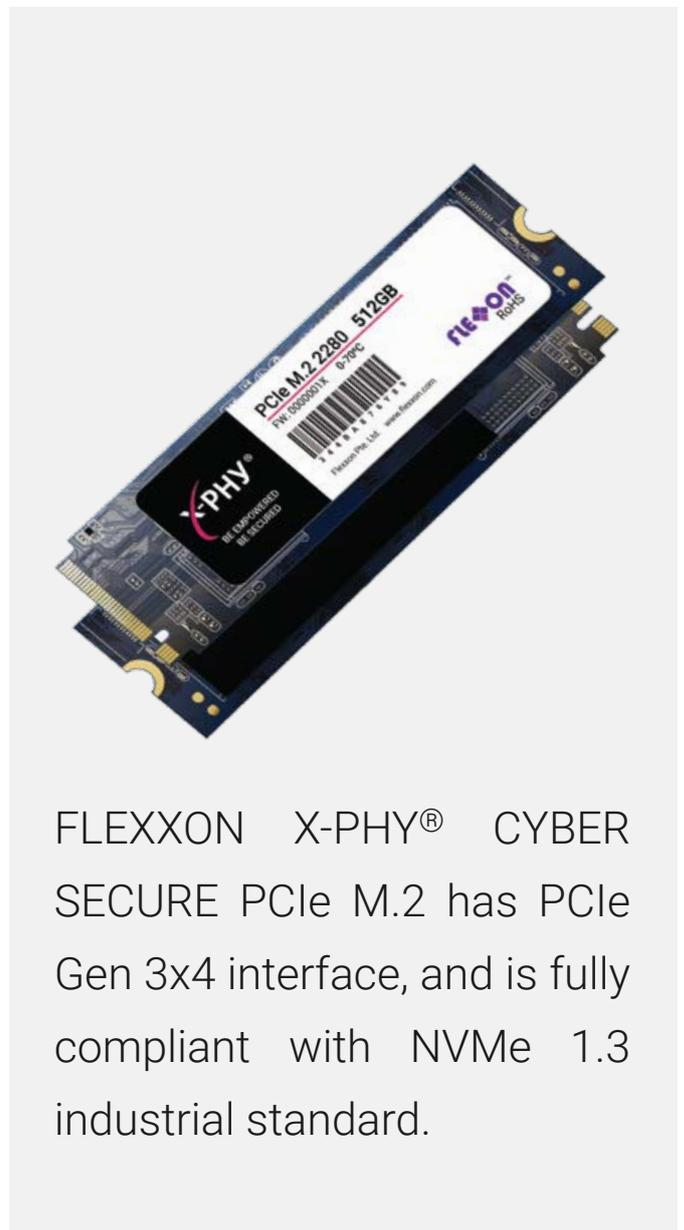
FLEXXON X-PHY® CYBER SECURE PCIe M.2 has PCIe Gen 3x4 interface, and is fully compliant with NVMe 1.3 industrial standard.
