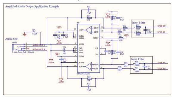
Further noise shaping can be employed by the addition of a DC blocking capacitor between the input filter and the input resistor of the audio amplifier. This forms a high pass filter which has a 3dB cut-off frequency described by the equation below.
