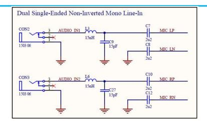
One 2-pole audio jack providing single mono audio source, unused inputs are AC grounded
