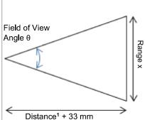
Note: The Recess value of 33 mm is the distance from the reader front face to the image sensor inside the reader. The Distance and Recess values are added together for the FOV Scan Area calculation.
