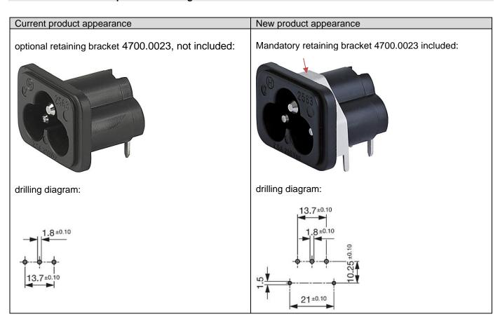
Retaining bracket is added as mandatory component. Before it was an optional accessory with part number 4700.0023.
