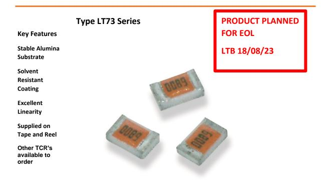
This thin film chip is manufactured by sputtering pure metals onto a high purity alumina base. This process ensures the element remains stable in performance over a long life. The LT73 is equally suited to temperature compensation or thermal protection when incorporated within the appropriate electronics. This range of sensors are finished in a tough epoxy seal and are available on tape for high speed auto placement.
