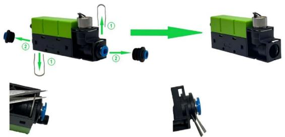
The metal ring for the rear fitting must be accessed from below.
