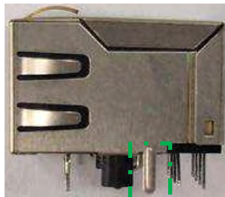
Above: Changed metal shield's pin from pre-plating process to pre-soldering process
