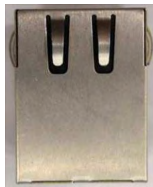
Above: EMI fingers are more curved for improved handling
