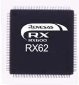
The **uEZGUI-RX621-35QT** includes a 100MHz Renesas RX621 or RX62N microcontroller running the open source uEZ® + FreeRTOS software platform. The RX62N has 512KB of internal Flash memory, 96KB of internal SRAM, a 10/100 Ethernet Media Access Controller (MAC), a USB full speed device/host/OTG controller, up to six UARTs, one CAN channels and a collection of serial communications interfaces. The unit also includes 512KB of external PSRAM.
