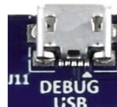
The J-Link® OB interface is multiplexed with the JTAG interface and can collectively be referred to as the Programming Interface. While the J-Link® OB interface and the JTAG interface do not conflict, the J-Link® OB signals may be isolated from the programming interface by changing the associated copper jumpers.
