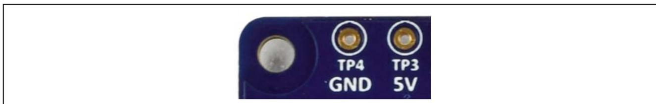
Figure 6. TP3 and TP4 on the Target Board
