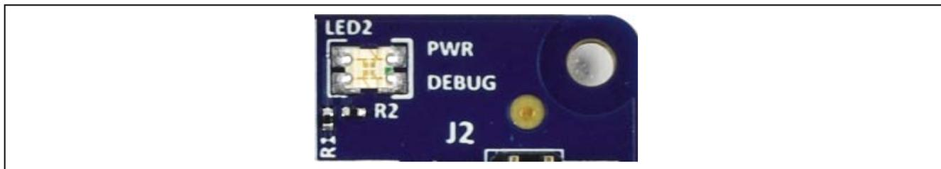
Figure 10. LED2 on the Target Board (Top Side)
