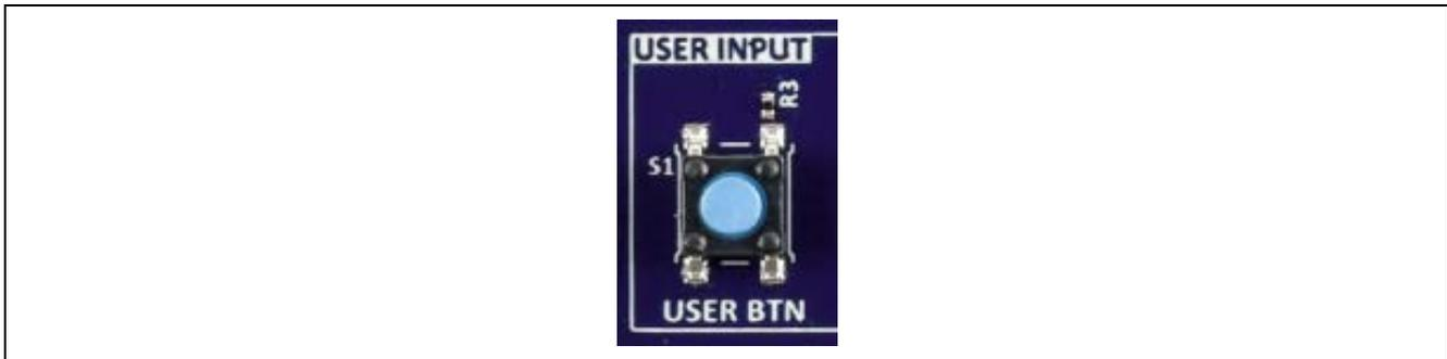
Figure 16. User Switch (S1) on the Target Board
