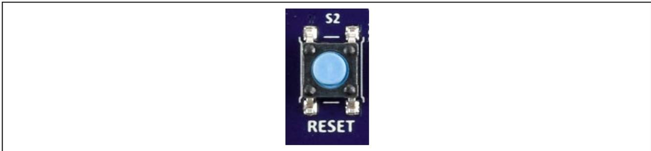
Figure 18. Reset Switch (S2) on the Target Board
