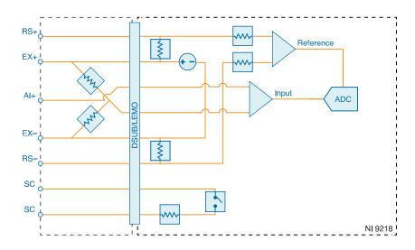
• The NI 9886 provides half bridge completion resistors for the incoming analog signal.
