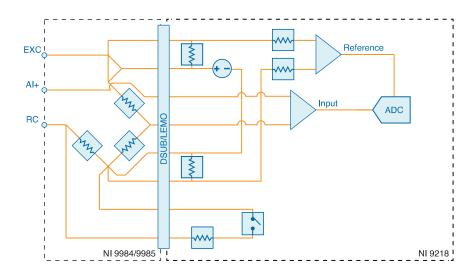
The NI 9984 and NI 9985 provide a quarter-bridge completion resistor and halfbridge completion resistors.
