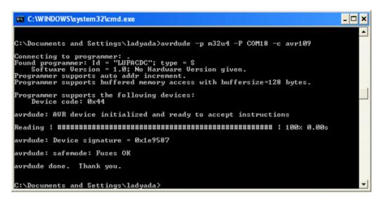
You can find the serial port COM# in the Device driver, or for mac/linux users run Is /dev/cu.usb\* to list all usb serial devices
