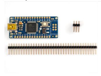
The breakout is almost completely assembled. We don't solder on the header or 6-pin ISP connector since we find it's easy to do but hard to undo, in case you want to put different headers on, or just connect up wires directly.
