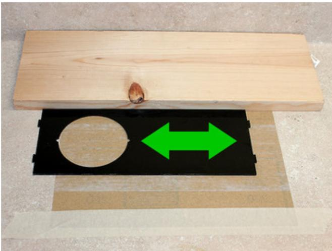
Here's the rig that was used to create the textured finish. A full sheet of 220 grit sandpaper (\$1.25) is taped face-up to the workbench, while a scrap of wood provides a straight edge to work against.
