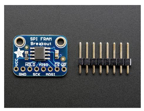
This particular FRAM chip has 64 Kbits (8 KBytes) of storage, interfaces using SPI, and can run at up to 20MHz SPI rates. Each byte can be read and written instantaneously (like SRAM) but will keep the memory for 95 years at room
