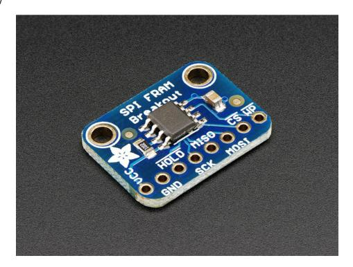
You're probably familiar with SRAM, DRAM, EEPROM and Flash but what about FRAM? FRAM is 'ferroelectric' RAM, which has some very interesting and useful properties. Unlike SRAM, FRAM does not lose the data when power is lost. In that sense it's a durable storage memory chip like Flash. However, it is much faster than Flash - and you don't have to deal with writing or erasing pages.
