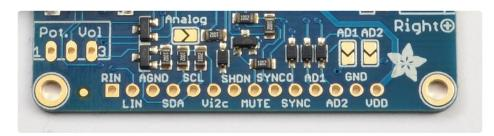
Above the pinouts there are three solder jumpers (Analog / AD1 / AD2) and then on the left, a 3-pin breakout called **Pot. Vol** - these are used in analog mode, the solder jumpers are closed to tell the chip we'll be using a potentiometer to set the volume. The **Pot Vol** connection is how we wire up the 1K potentiometer. This is covered in more detail in the Analog Wiring section.
