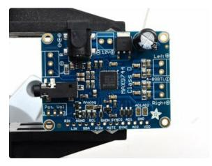
Place the capacitor against the PCB and bend the two leads out so that it sits flat.
