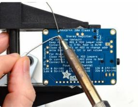
Solder in both pads, heating the pad and pins at the same time with the edge of the soldering iron and dipping a little solder in.
