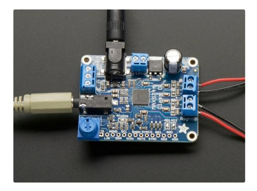
Once you have that working, you can solder wires to the **Pot Vol** pads, so you can place the volume adjustment pot elsewhere (say mounted to the outside of a box)
