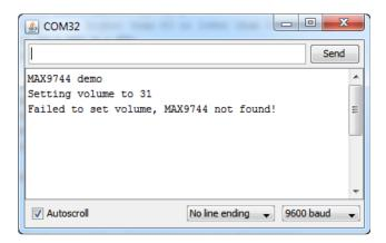
If it's OK, you can send multiple +'s and -'s to increase or decrease the volume. The volume can go down to 0 or up to 63 (which is 29dB of gain)
