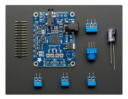
Each order comes with one MAX9744 breakout board with all surface-mount parts fully assembled and tested. We also include 3 x 2pin and 1 x 3pin terminal blocks, a 470uF power filter capacitor and 1K $\Omega$  trim pot. To use this board, a little soldering is required to attach the terminal blocks and other components, but its fairly easy and expect it should take less than 15 minutes.
