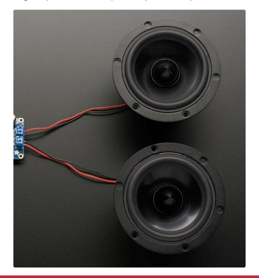
Don't forget to gently yank on each wire after clamping it into the terminal block, it should be a solid connection, not possible to yank out of place. Loose wires will be a problem!
