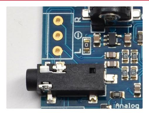
The headphone jack is a classic 3.5mm as seen in just about every audio device. You can connect this directly to any audio output. The terminal blocks are for if you have some direct-wiring project and you want a more permanent connection. You'll have to solder in the terminal blocks if you want to use that technique, see the Assembly page
