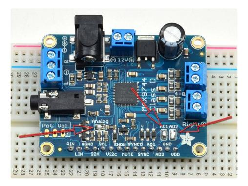
When you power up the amplifier and feed in audio you won't hear anything! This is normal! If the potentiometer is not installed, it will default to lowest volume.
