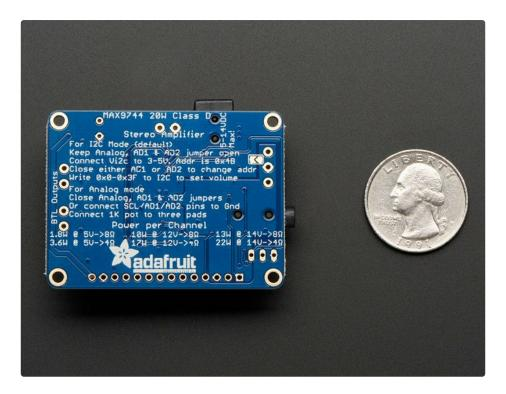
We like the MAX9744 amplifier at the heart of this board because its very easy to use, but it also has *both* analog and digital volume control capability. Use a single 1K  $\Omega$  pot (we include one) to adjust volume analog-style. Or hook it up to your favorite microcontroller and send I2C commands to set 64-steps of volume amplification.
