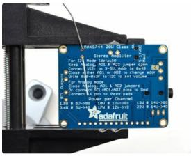
Flip over the board so you can solder the two pads
