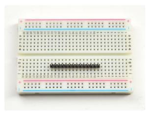
Break off a piece of 0.1" male header, 14 pins long and stick it long pins down into the solderless breadboard
