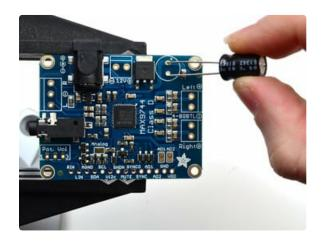
Capacitors are polarized, they have to be placed in the right way!
