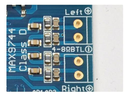
The speakers can be 4 to 8 ohm impedance, 20W maximum power. Since it is a class D amplifier, the signal out of these speaker blocks is a high frequency (~300KHz) PWM square wave. The inductance of the speaker smooths out this signal into audio frequencies of 20-20KHz.
