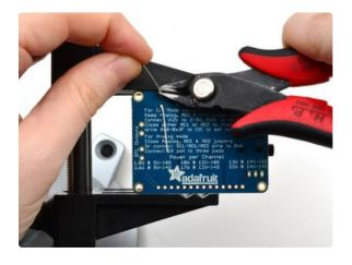
Clip down both of the long leads using diagonal cutters so they are nice and neat
