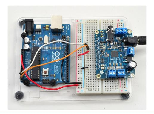
Make sure the AD1 AD2 and Analog solder jumpers are not closed before running the I2C tests, or it won't work! For digital mode, these jumpers must be un-soldered
