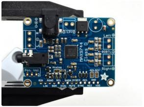
Begin by placing the amplifier board in a vise so you can easily work on it. Heat up your soldering iron to 650-700 degrees F and get some solder and hand tools ready!
