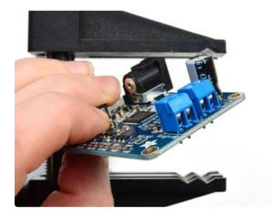
Place two of the 2-pin blue terminal blocks so that the holes point outward
