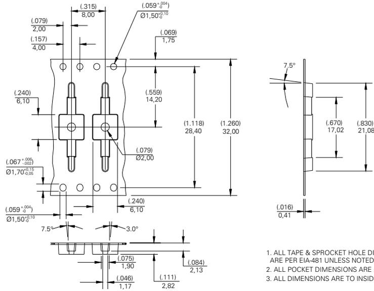
1. ALL TAPE & SPROCKET HOLE DIMENSIONS ARE PER EIA-481 UNLESS NOTED
