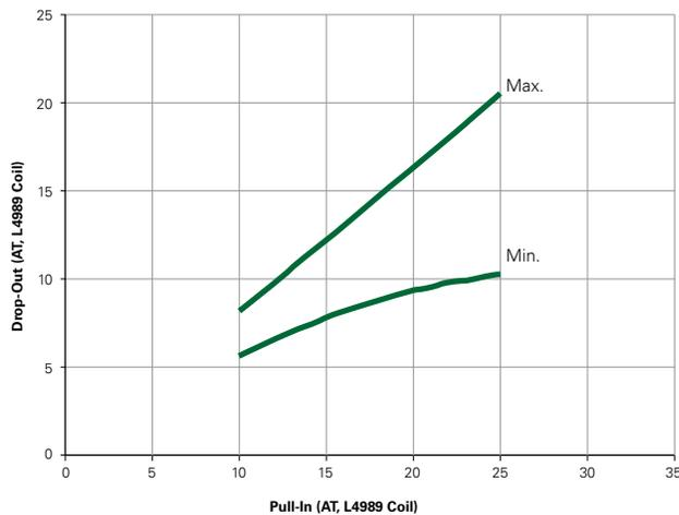
**Note:** Chart represents the range of Drop-Out, min to max, for a given Pull-in value of the MDSR-10 prior to modification into the MDSM-10.
