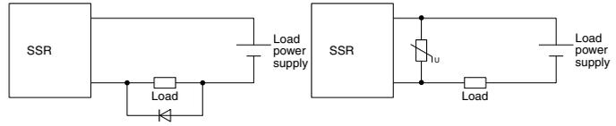
3) Clamp diode and snubber circuit can limit spike voltages at the load side. However, long wires may cause spike voltages due to inductance. It is recommended to keep wires as short as possible to minimize inductance.
