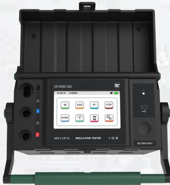
*STI Insu 5Dt* is a 5KV Digital Insulation Tester with selectable test voltage upto 5KV and Insulation Resistance measurement upto 2 T $\Omega$ . Ideal for insulation testing of cables, motors and transformers. It comes with a facility to measure PI, DAR, Step Voltage, Ramp test.
