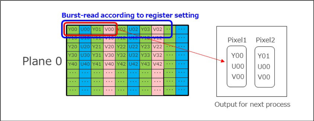
Figure 36.4 Example of Interleave Format for YCbCr422 (YUV422)
